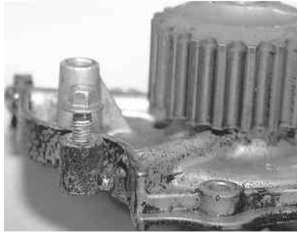
Fig. 3: Make sure the water pump O-ring is fully seated in the water pump. Using a non hardening gasket sealant will help to hold the seal in place during assembly
